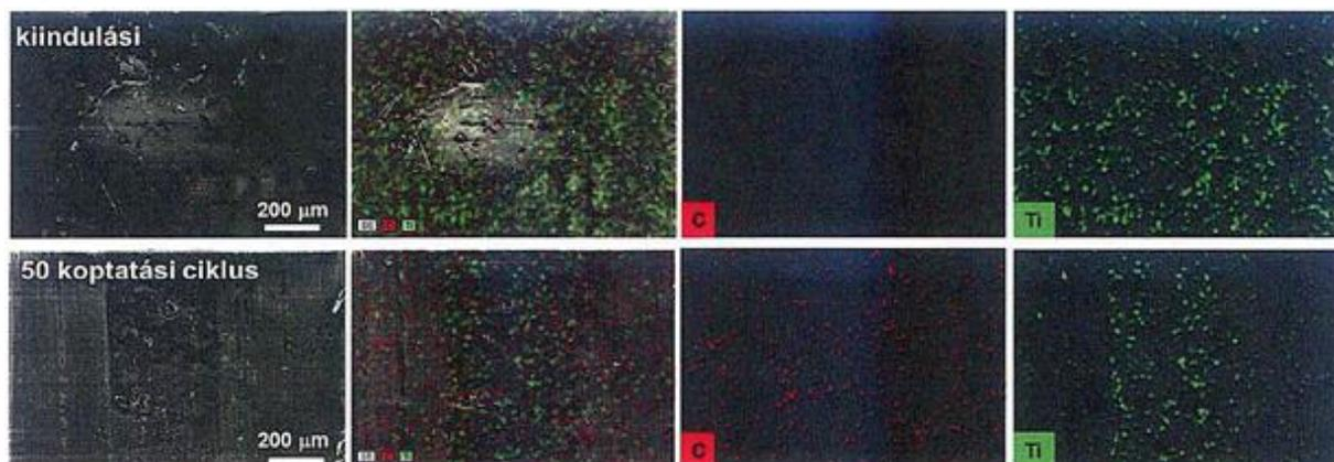
Figure 6. After the initial and 50 abrasion cycles, the element distribution of the composite films (indicating the presence of carbon (red C) and titanium (green Ti)) on the glass substrate surface
