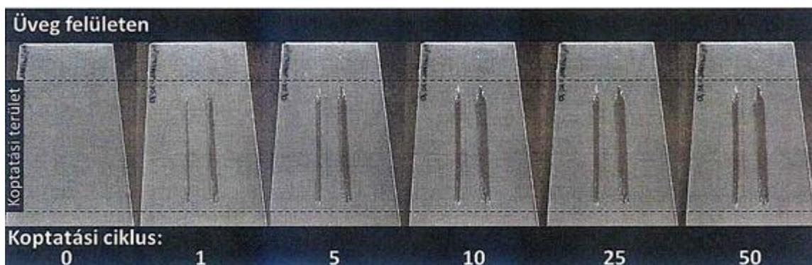
Figure 5. Photograph of composite (photocatalyst / polymer) films on glass substrate after 0, 5, 10, 25 and 50 abrasion cycles
