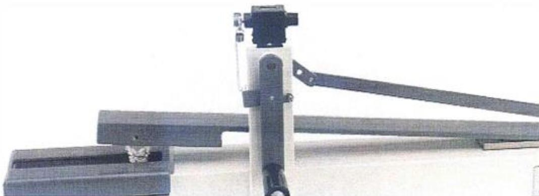
Figure 1. Photo of a crockmeter.
