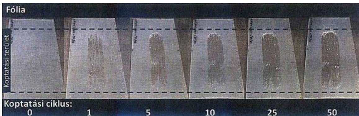
Figure 4. Photograph of composite (photocatalyst / polymer) films formed on a film support after 0, 5, 10, 25, and 50 abrasion cycles.
