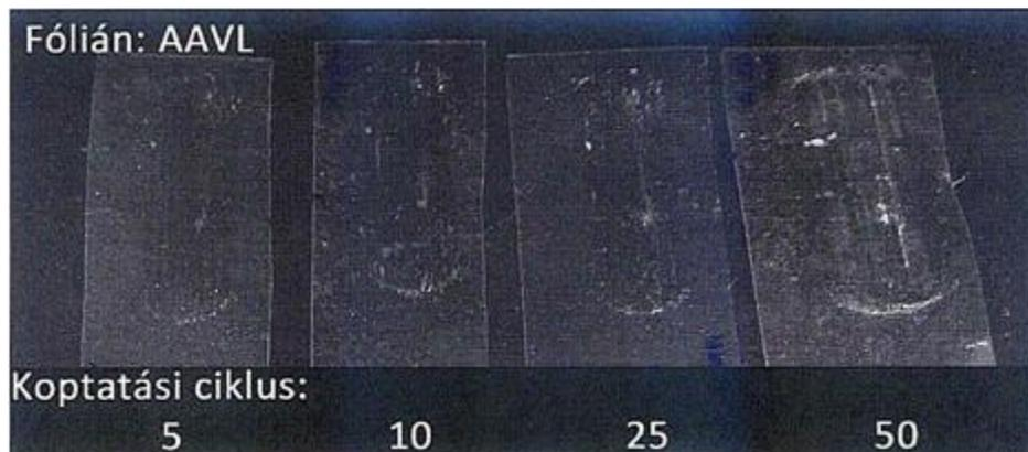
Figure 2. Photograph of films formed on the film-carrier polymer (AAVL) after 5, 10, 25, and 50 abrasion cycles.
