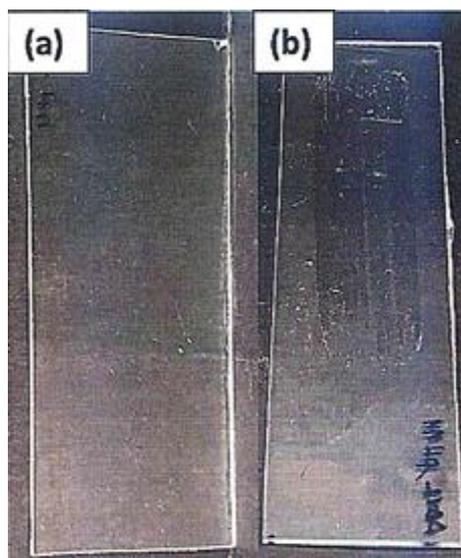
Figure 3. Photograph of the polymer film after the initial (a) and 50 abrasion cycles formed on the glass substrate.
