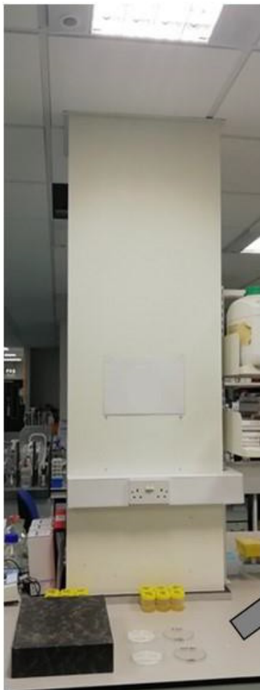
Figure 1 A: Schematic of test assembly described within BS ISO 27447:2019; B: Photograph of the test assembly used for analysis of Resysten samples.
